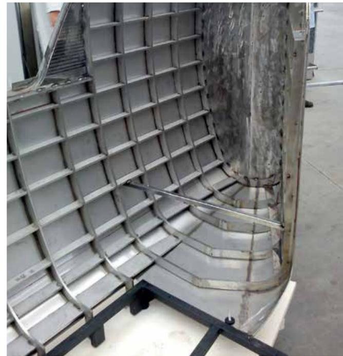
■ Above left: axonometric structure, elevation and plan of the reception desk at the Al Mourjan business lounge. Below: the same reception desk as seen at the airport. Above right: the construction process of one of the steel check-in counters
